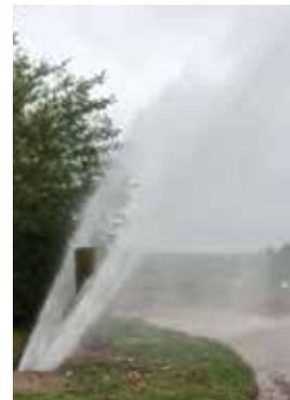
By deploying the leading data analytics suite - InflowSys™, high resolution pressure data was captured and analysed in real time to identify transient sources and dynamic pressure variability causing network asset fatigue and hence burst failure. The asset fatigue was measured using the InflowSys™ Cumulative Pressure Induced Stress index (CPIS™) in order to prioritise future potential at risk areas.
